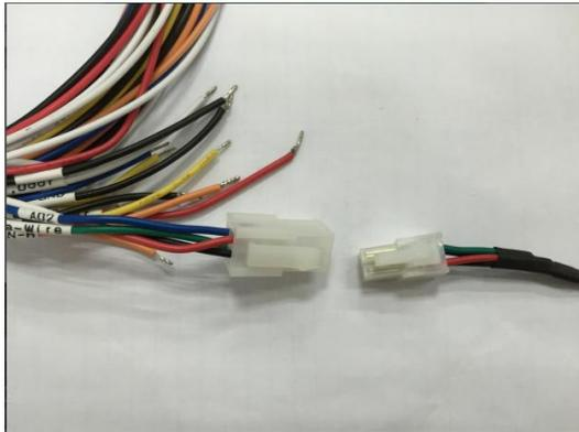
According to the above figure, the white interface on the left is the tracker's dedicated port for a temperature sensor and fuel level sensor, and the white interface on the right is the iButton reader's connector.
