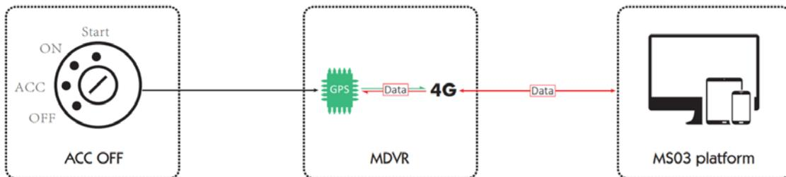
As shown in the preceding figure, the video system stops operating, while the vehicle tracking system is operating.
