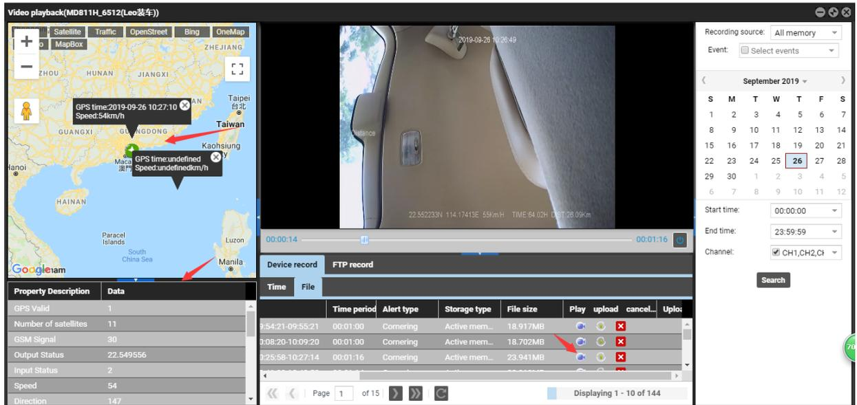
While playing back video files, the location information of related images will be displayed and travel routes will be played. As shown in the previous figure, the icon in the **Play** column is used to play the current video, the icon in the **Upload** column is used to upload the current video file to the FTP server, and the icon in the **Cancel** column is used to stop uploading the video file.
