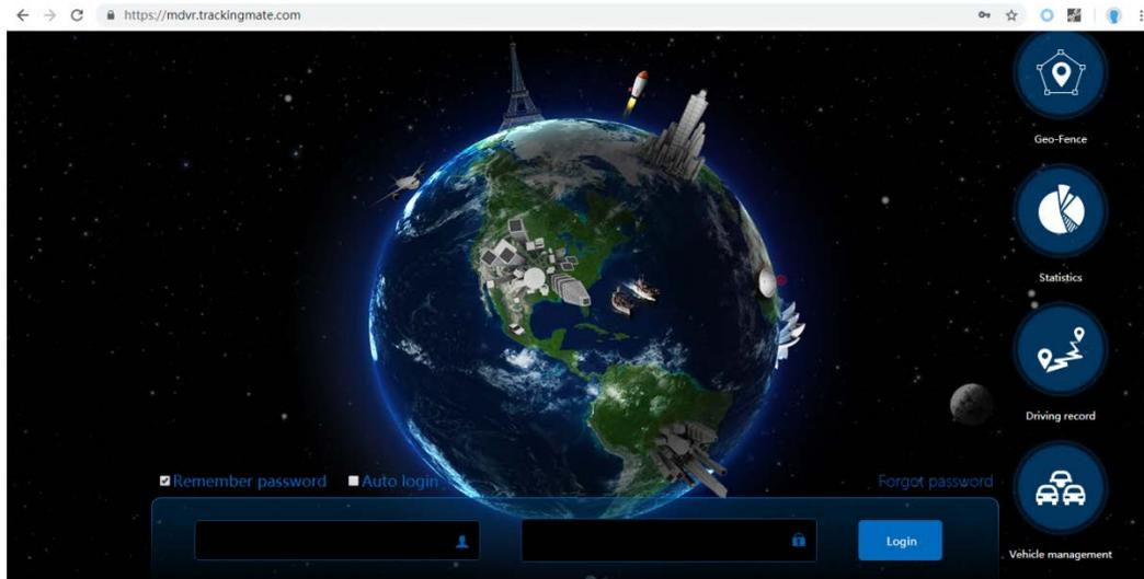
After logging in to the platform and adding the MDVR, you can use the positioning function, monitor the MDVR in real time, play back videos, query alert videos, and make a call.
