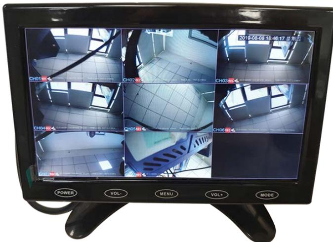
Note: There are two types of displays available, that is, the display with an AV-OUT interface (CVBS display) and the display with a VGA interface (VGA display). Users can select one or two displays as required.
