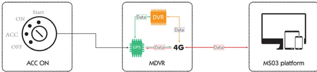
As shown in the preceding figure, the video system and vehicle tracking system operate simultaneously.
