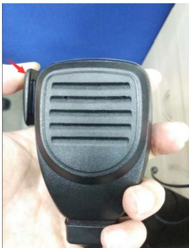
Before a talk starts, MDVR users need to press and hold down the talk button at the left side of the MDVR. During broadcasting, a call can be made between platform users and MDVR users, while MDVR users cannot talk with each other.
