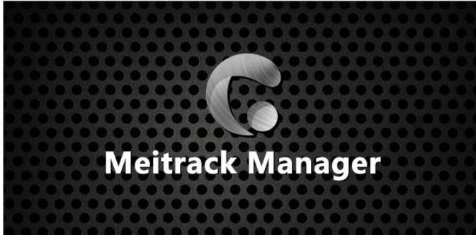
You need to install Meitrack Manager first. (Visit [www.meitrack.com](http://www.meitrack.com) to download the software). After the installation is completed, connect the USB cable to a computer, and then perform the following steps to configure the MDVR.
