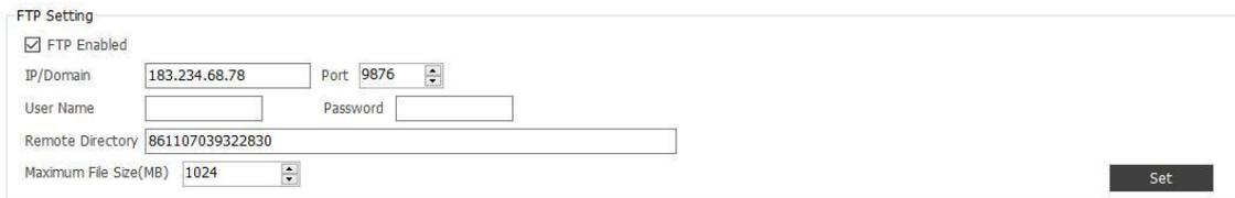
The screenshot shows the 'FTP Setting' configuration window. It includes a checkbox for 'FTP Enabled' which is checked. Below it are input fields for 'IP/Domain' (183.234.68.78), 'Port' (9876), 'User Name', and 'Password'. There is also a 'Remote Directory' field with the value '861107039322830' and a 'Maximum File Size(MB)' dropdown set to '1024'. A 'Set' button is located at the bottom right of the form.
