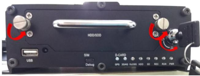
Open the disk cover by using a screwdriver, and then install a disk.
