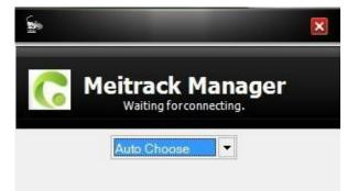
4. Turn on the device, then Meitrack Manager will detect the device model automatically and the parameter page will appear accordingly.
