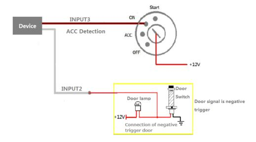
Note: If input 3 is connected to the "ACC" position, after the engine is started, the platform will read it as ON-OFF-ON. If input 3 is connected to the "Start" position, after the engine is started, the platform will read it as OFF-ON-OFF. If installed correctly, after the engine is started, the platform will read it as OFF-ON.
