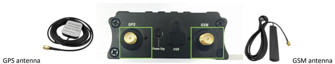
Connect the GSM antenna to the connector which is labeled "GSM". The GSM antenna is non-directional, so you can hide it in any place of a vehicle.
