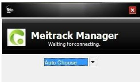
4. Turn on the device, then Meitrack Manager will detect the device model automatically and the parameter page will appear accordingly.
