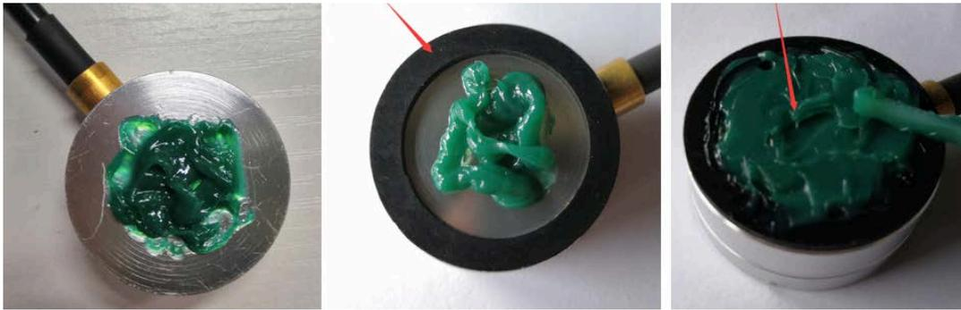
Insert the sensor into the holder and install the cover plate.
