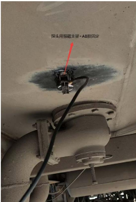
If the ambient temperature is 25°C, move the probe for 30 seconds after sticking the probe. In this way, if the result is unable to install, remove the probe, clean up all AB glue, and apply glue to the probe surface again. Because the AB glue does not work at this moment.
