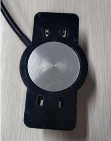
Stick the probe on the marked location and check the app result is ok or invalid. If no, move the probe slowly within 2–3 mm and find the right installation location.
