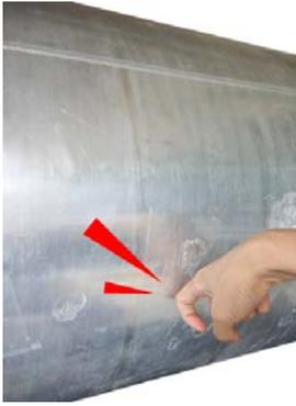
When there is fuel in the fuel tank, you can hear a muffled sound.
