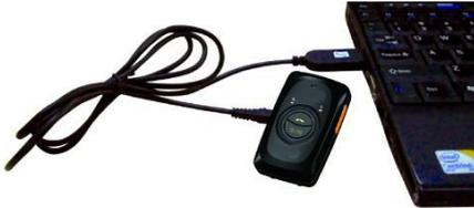
For the T1/T333/T622, after the device is connected to the computer, you need to press and hold down the power button for 3 seconds to turn on it. For the MT90G/MT90/TC68S, the device will turn on automatically upon connecting to the computer. You are advised to turn off the device if you do not use it after parameter settings.
