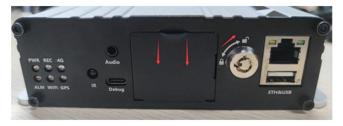
(2) Install the SIM card and SD card, and then lock the SD card lock back. (Note: After closing the card cover, you need to lock it with the key to ensure that the video function starts normally)
