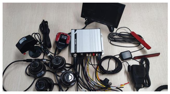
Connect the power cable to PWR Connect 1~6 cameras to AV IN1~IN6 Connect the display to AV-OUT/VGA Connect the intercom handle to MIC&SPK Connect WIFI antenna (otherwise you can't use WIFI properly), GPS antenna, 3G/4G antenna
