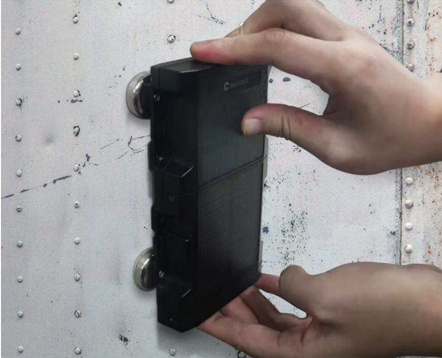
The following figure shows how to install the tracker onto a truck:
