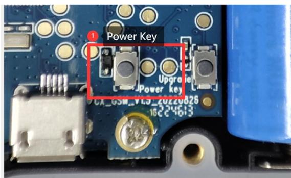
Hold down the power button for 3 seconds and the device will shut down.
