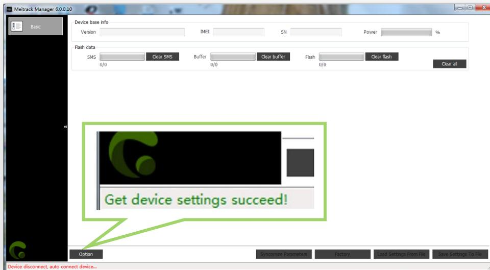
Note: If the connection fails, check whether the USB driver is installed.
