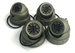
The mobile DVR supports up to 2 TB storage capacity. Inside each school bus, a mobile DVR is connected to four cameras for live video surveillance, and videos can be stored for one month (six hours per day). The cameras can even operate in a more than 80°C ambient temperature and features the IP67 water resistance rating.
