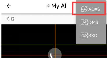
2) Adjust the position of the yellow and red lines in the picture by hand, placing the red line at the level of the road and the vertical orange line at the point where the road ends.
