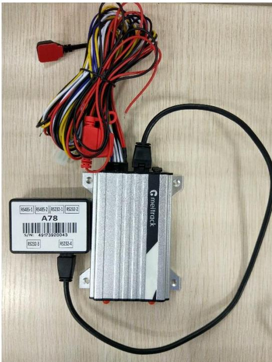
Connect the A78 to two cameras, two A82 seven-segment digital displays and a magnetic card reader:
