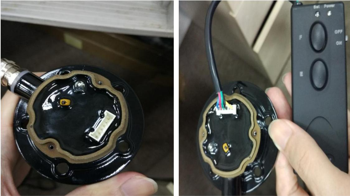
2. Calibrate the full level: Fill the fuel tank to the full level, put the sensor into the tank, and wait for about 30 seconds until the sensor tube is filled with fuel. Then press and hold down the **F** button of the calibrator. The sensor will enter the full level calibration mode if the green LED indicator blinks. Then release the **F** button. After about 10 seconds, the full level is calibrated successfully if the green LED indicator is off.
