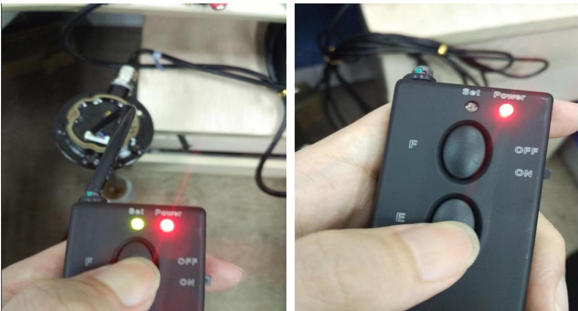
3. After calibration is finished, disconnect the calibrator, close the sensor cover, and tighten the screws. Then connect the red and black cables to the tracker's power cables. The calibration will become effective after the sensor is powered on.
