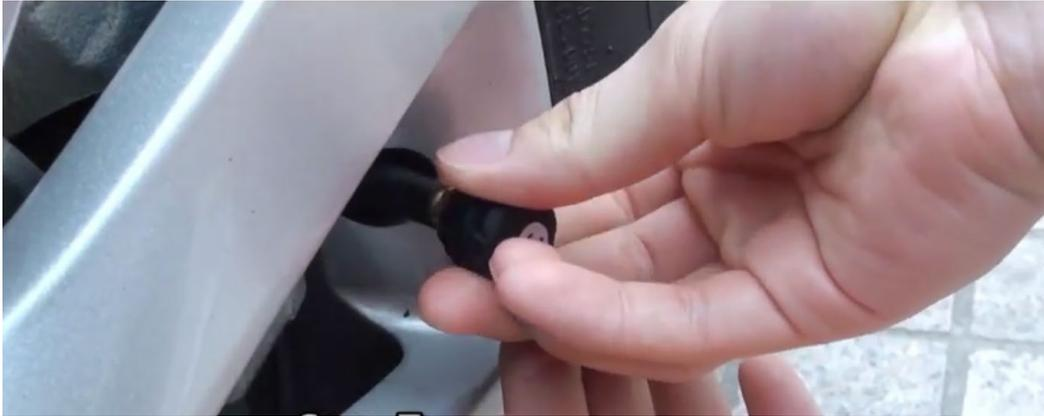
(4) Use a fixture to tighten the anti-theft nut counterclockwise to prevent theft of the tire pressure sensor.
