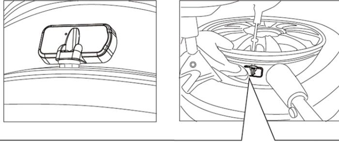
Remark: please hold on the sensor by hand, so that the sensor position can not be changed when the screw nut is mounted.
