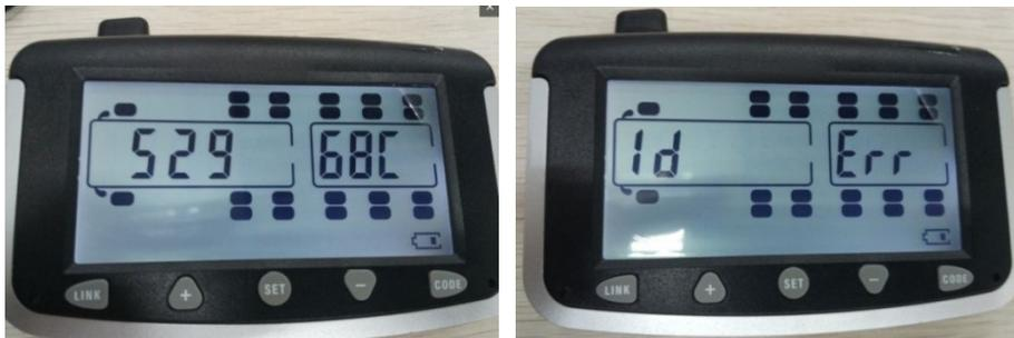
When the corresponding wheel is selected, the appearance of the ID number indicates successful pairing. If 'ID ERR' appears, it indicates pairing failure and requires re-operation.
