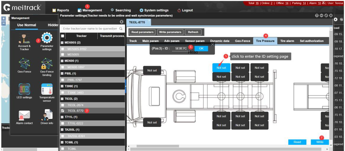
As shown above, the tire pressure sensor with ID 5E0E7C is bound to the second tire at the vehicle front. After binding the vehicle front tires, dragging the navigation bar allows entry to the tire binding interface for Card Slot 1; further dragging grants access to the tire binding interfaces for Card Slots 2, 3, and 4. The configuration method for the card slots is the same as for the vehicle front.
