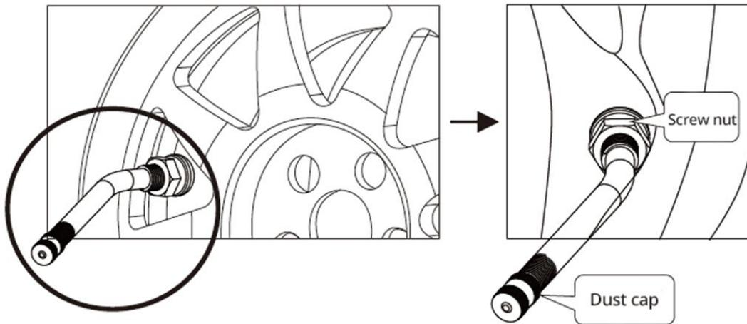
(5) After completing the installation, re-inflate the tire to the specified pressure, then conduct dynamic balance testing.
