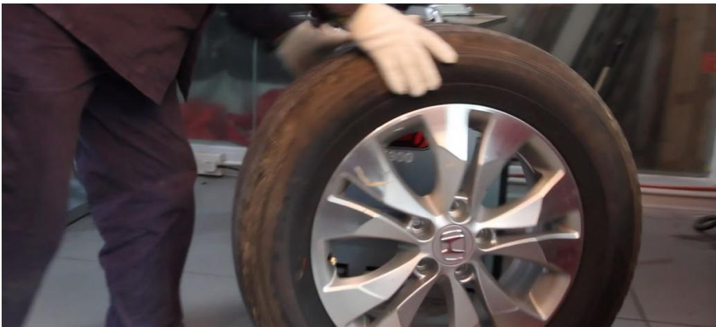
(3) After prying open the tire, use a knife to remove the original valve stem:
