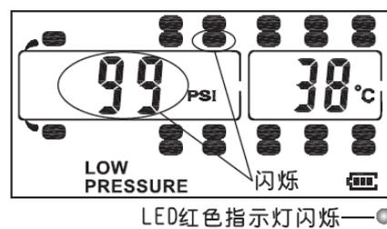
High Pressure Alarm: The red LED and the corresponding tire will flash.
