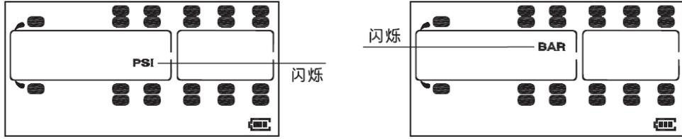
Press the + or - key to select the desired pressure unit.
