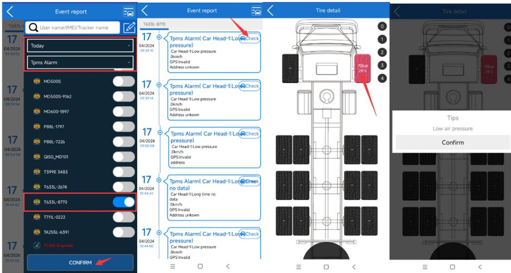
**Note:** Clicking 'Check' will open the tire pressure information page, where red indicates an alarm and black indicates normal status. Clicking on the color will display the specific alarm type.
