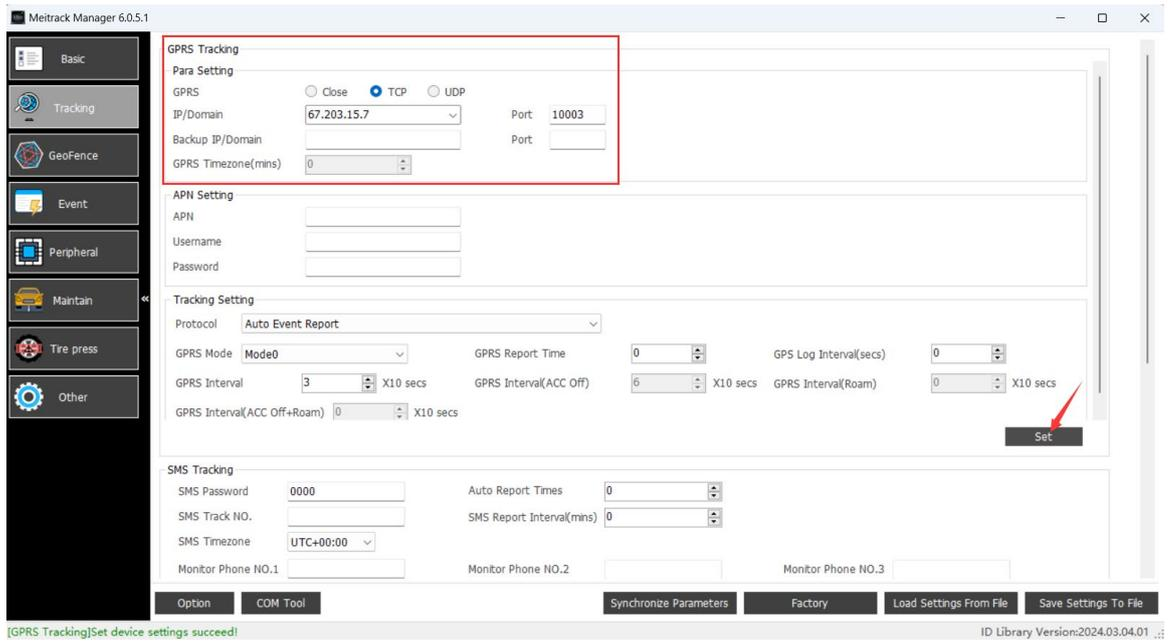
(2) Configuration can commence once the platform indicates the device is online. The settings interface and procedure on the MS03 platform are identical to those in Meitrack Manager. The detailed settings interface is illustrated below:
