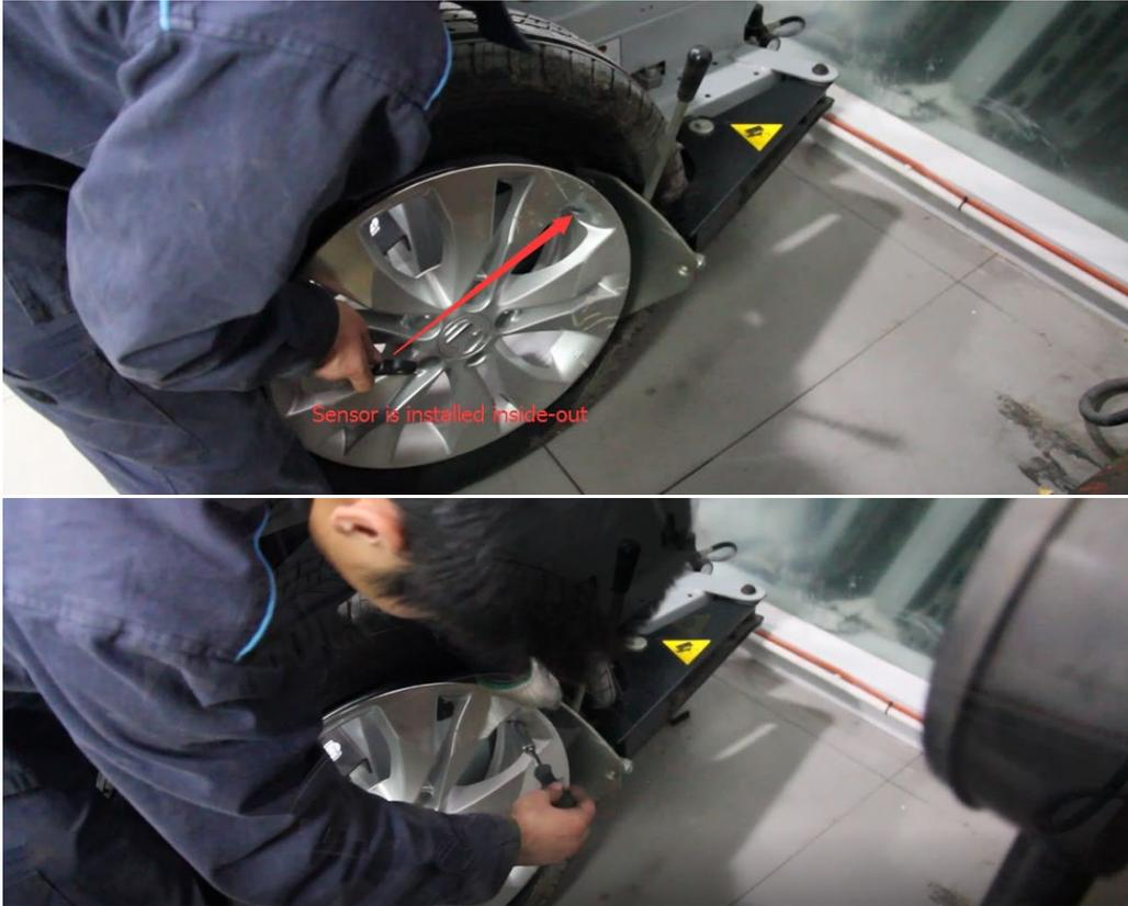
The structural installation schematic is as follows: the wing head faces inward, the valve stem faces outward, and the nut is fastened simultaneously:
