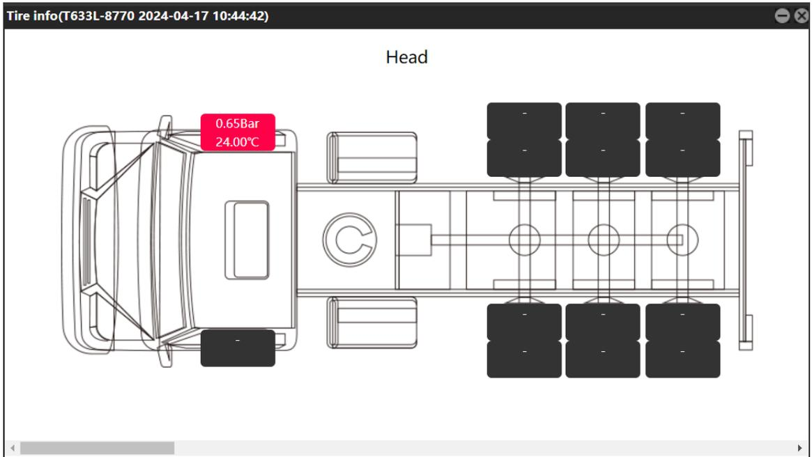
Hover the mouse over the corresponding tire location to display the specific alarm type, such as 'Low Tire Pressure' or 'No data received for an extended period.'
