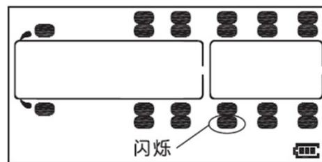
Sensor Low Battery Alarm: LED red light and corresponding tire flashing
