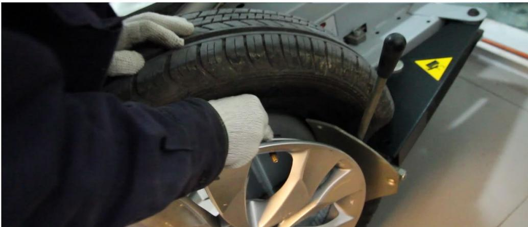
(4) Install the sensor wing and valve stem assembly, then securely tighten:
