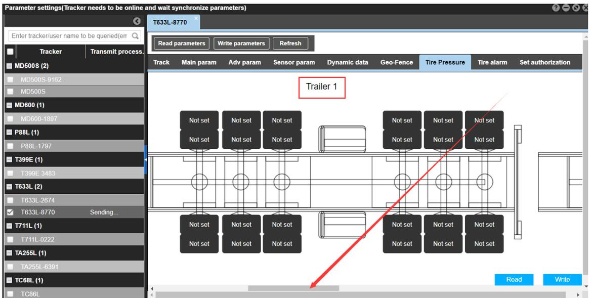
(3) After binding the tire ID, it is necessary to set the alarm value. Click “Tire alarm” to access the alarm value setting interface, as shown below:
