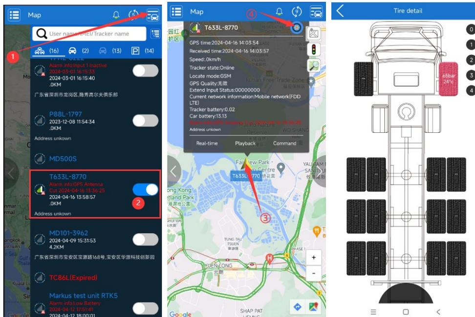
(3) Bind the Tire Pressure Sensor ID. Enter the sensor ID corresponding to the tire location to bind the tire pressure sensor to the tire. To switch to another cartridge, simply tap the numeric navigation button on the right side of the screen. For example, tapping button “4” will switch to cartridge 4.
