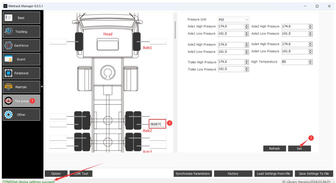
(3) Since the vehicle front is particularly important, alarm values can be set individually for the four axles' tires at the vehicle front. These alarm value settings are located at the upper right corner of the interface. Tire pressure values can be displayed in two selectable units: 'PSI' and 'bar'.
