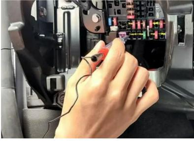
2. If you do not know which fuse socket corresponds to the turn signal, please use a multimeter or test pen to measure, as follows:
